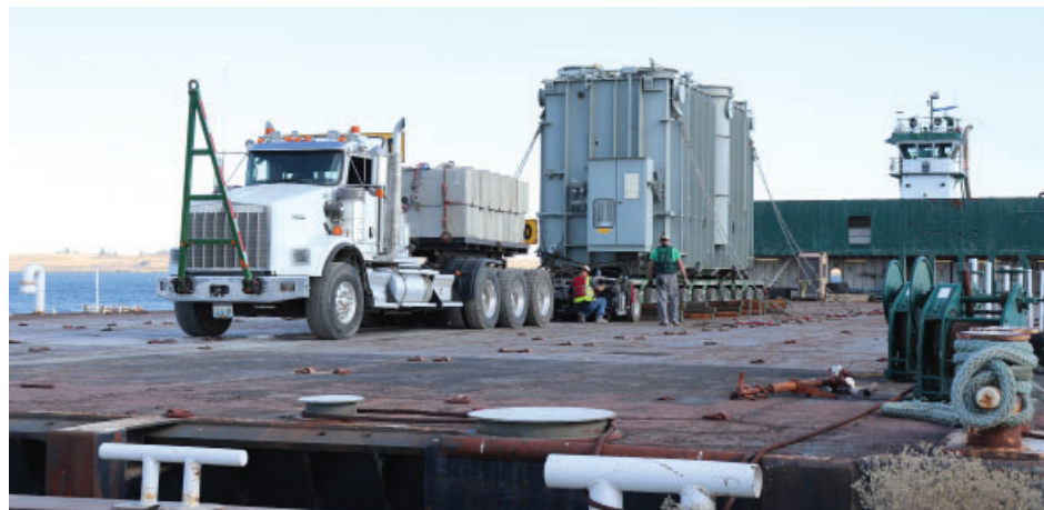
August 2019: Omega Morgan transferred a 507,000-pound transformer from the Coyote Springs Power Plant in Boardman to a barge for transport to Vancouver, Washington where it would meet a ship to carry the transformer overseas.
